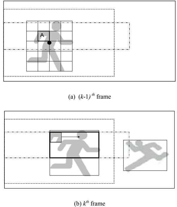
Fig. 4. Template matching process
