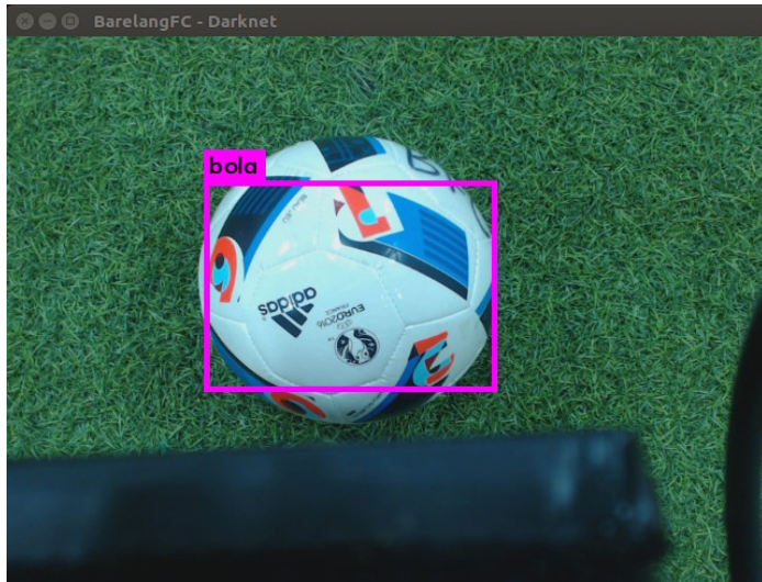
Fig. 6 Ball detection in less lighting condition.
