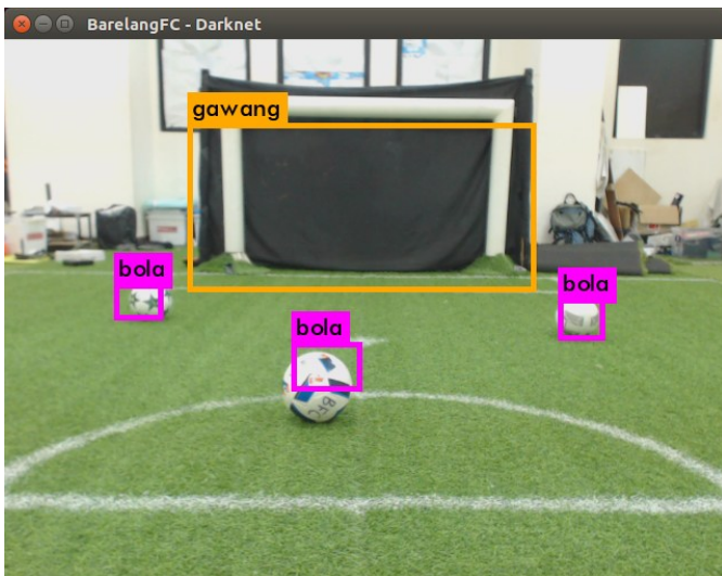
Fig. 11 Ball and goal detection covered by black fabric.
