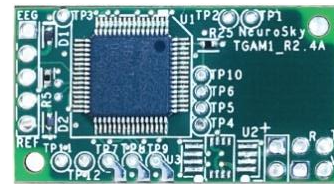
Gambar 2.2 NeuroSky Brainwave Sensor (TGAM)
